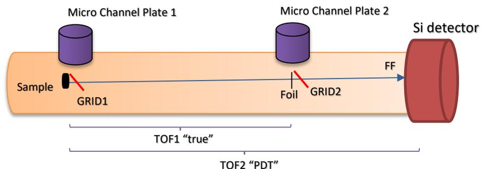
**Fig 2: The setup used for the plasma delay time studies, at the TANDEM facility in Ångström lab.**
